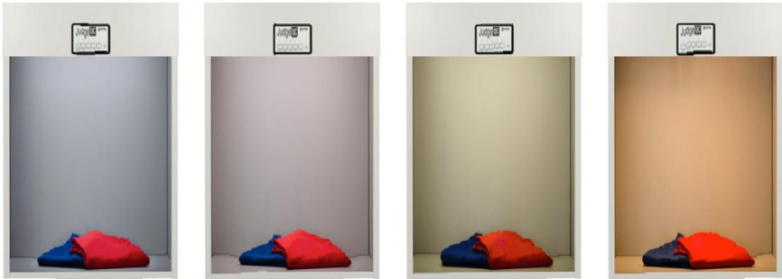
Figure 7. Illuminant metamerism due to the change on different SPD, CCT, CRI, Lux [197]
