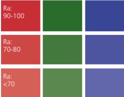
Figure 27. Colour rendering index (CRI) and temperature [201]
