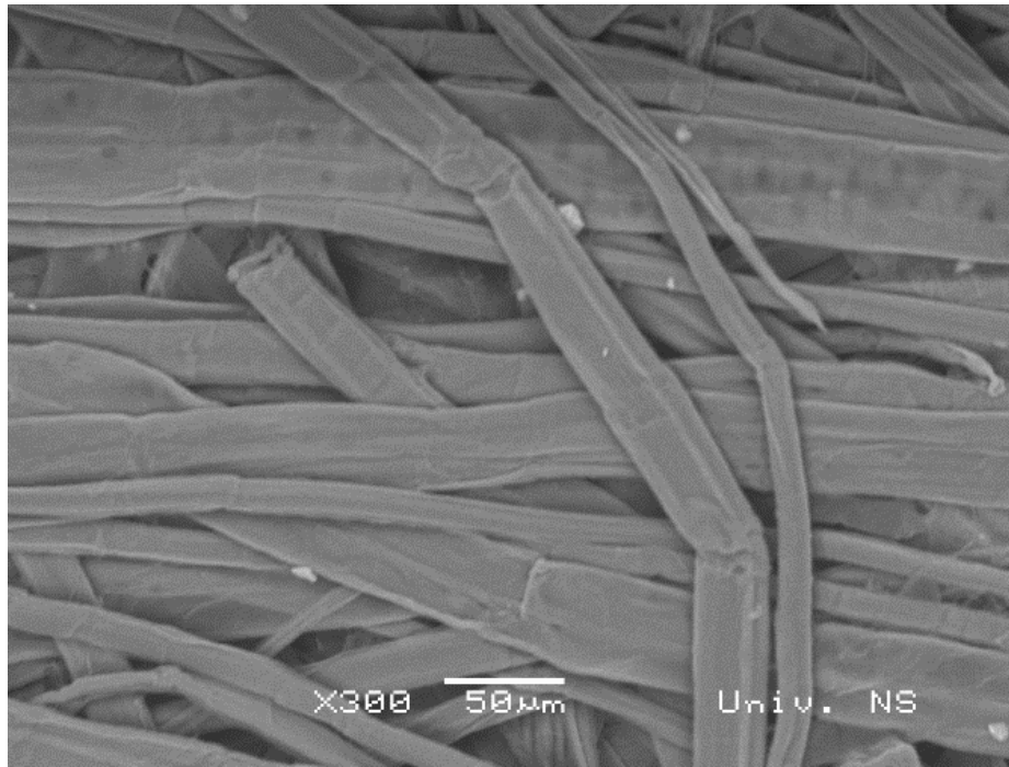
Figure 3 - SEM micrograph showing the surface morphology of the model paper at 300× magnification.
