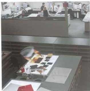
Fig. 1.2-24 Prepress with conventional film stripping and digital master preparation (text, images, graphics) with EDP systems
